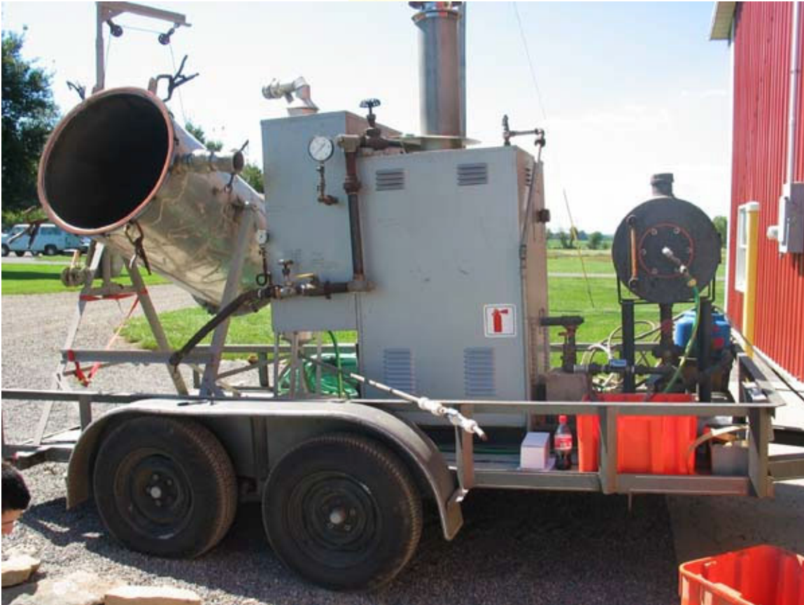
Figure 4 - The portable steam distillation unit used in the present work. The distillation tank (left) is tilted to facilitate loading/removal of plant material. The system has a series of pressure regulators to monitor and maintain pressure. Photo taken while preparing the unit for this study, Pittstown, New Jersey.
